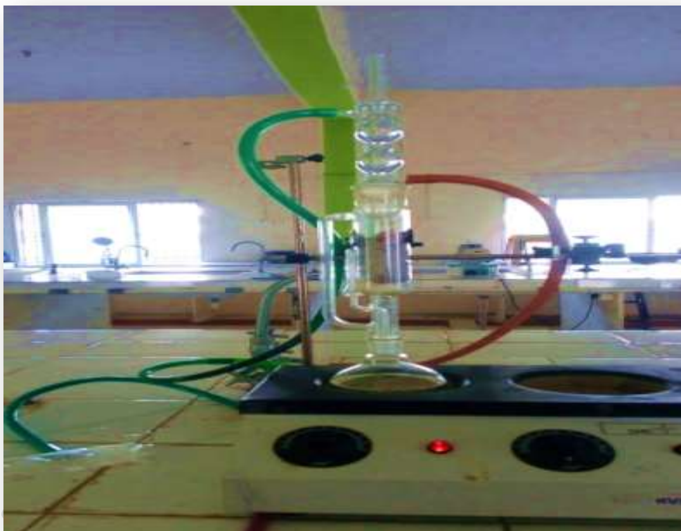
Figure 3: Aqueous Extraction of Pulverized green tea leaves.
