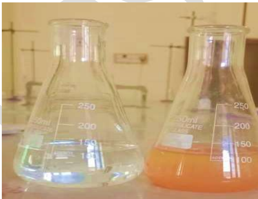
Figure 4: Synthesis of Ag-NP (Silver Nanoparticles) from reaction between AgNO_3 and green tea extract.
